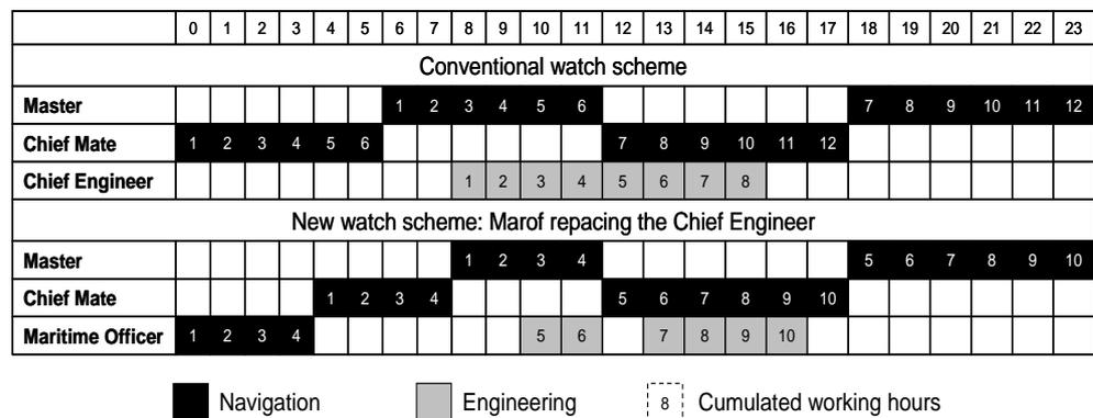
Figure 3-1 Watch schedules for two different manning concepts. The columns represent the hours of the day; the rows the crew. Black cells show navigation hours, grey cells engineering hours. The numbers in the cells represent cumulated working hours within a day.
