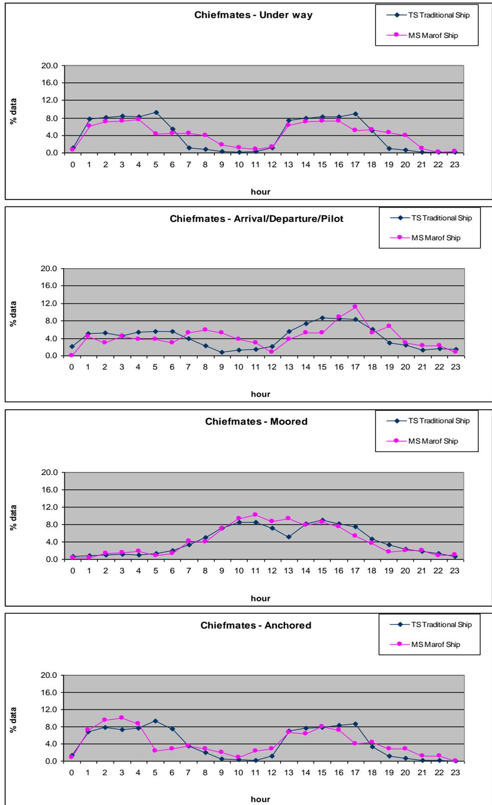
Figure 4-13 % watch hours of the Chief Mates, divided over the 24 hours of a day, at the Traditional and Marof ships, and shown for the four voyage phases.
